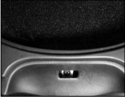
STEP 22: With OEM outer console, OEM inner cut console and hinged lid mounted. Look in the lid latch catch, located on the front of OEM inner console. You will see the small angle bracket that was mounted in STEP 11 . Drill 1/8" hole through the lid latch catch using the hole from the small angle bracket as a guide. Mount the small angle bracket with supplied #8x1/2" black pan head screw to the Stealthbox.
